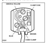
Connect the Green and Yellow (earth) wire to the terminal in the plug which is marked with the letter «E» or the earth symbol (a) or coloured green and yellow.
